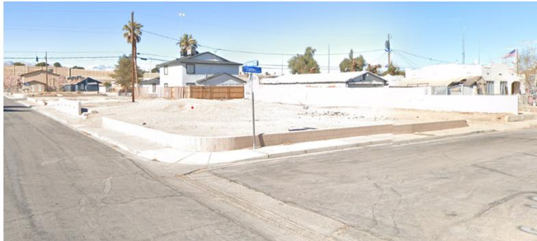
The proposed site currently has drive access from both Oxford Avenue and Stanford Street. The existing vehicle access from Oxford Avenue is not proposed for use, while the access from Stanford Street will need to be enlarged as the main drive access for the property. It is currently a single
